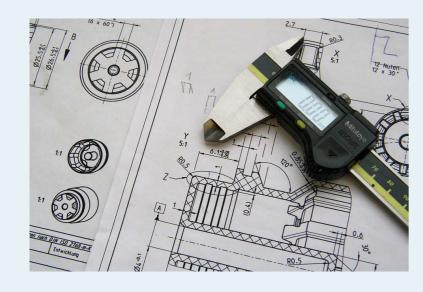
**Scale** informs the engineer what scale should be used when using the drawing. A scale of 5:1 indicates that the drawings are five times smaller than the original product should be. This allows engineers to take dimensions (sizes) directly off the engineering drawings. Care must be taken when doing this to ensure the correct scale is applied.
